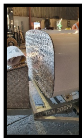
Front aluminium checker plate stone guard
