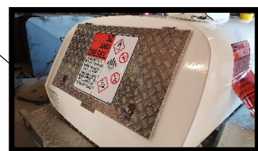
Rear access door to pump bay made from aluminium checker plate with double lockable latch system
