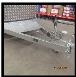
Galvanized chassis with tandem axle and hydraulic braking system on front axle.
