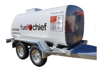
The Fuelchief Trailer Tank FCTT1900 is a single-skin 1,900L diesel storage tank built to transport fuel on public roads and highways, as well as refuelling to construction sites. The tank's lockable pump bay positioned at the rear of the tank provides secure and easy access for fuelling.
