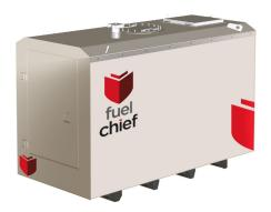
The DC Series is a robust tank designed with no internal bracing. The smallest in the series is the **DC25**, ideal for SME operations or as a back-up tank for generators and pumps. The DC25 provides 110% secondary containment while the full height internal pump cabinet makes it ideal for security and quick refuelling.
