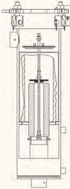
Vel-Max Series for liquid/liquid separation uses a 2-stage coalescer separator cartridge combination to remove free and emulsified water from a liquid product stream. The first stage coalescing cartridge provides filtration as well as coalescing of free and emulsified water. The second stage separator is a hydrophobic barrier designed to repel the coalesced water droplets. The water droplets will fall and collect in the sump for removal through the manual drain.
