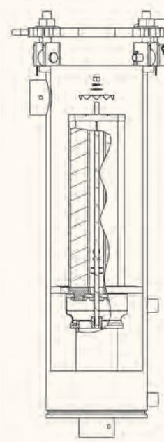
Vel-Max Series can be adapted to use 2" diameter CDF® type monitor cartridges\* for removing solid contaminants and free water by absorption from jet fuel or aviation gasoline flow streams.
