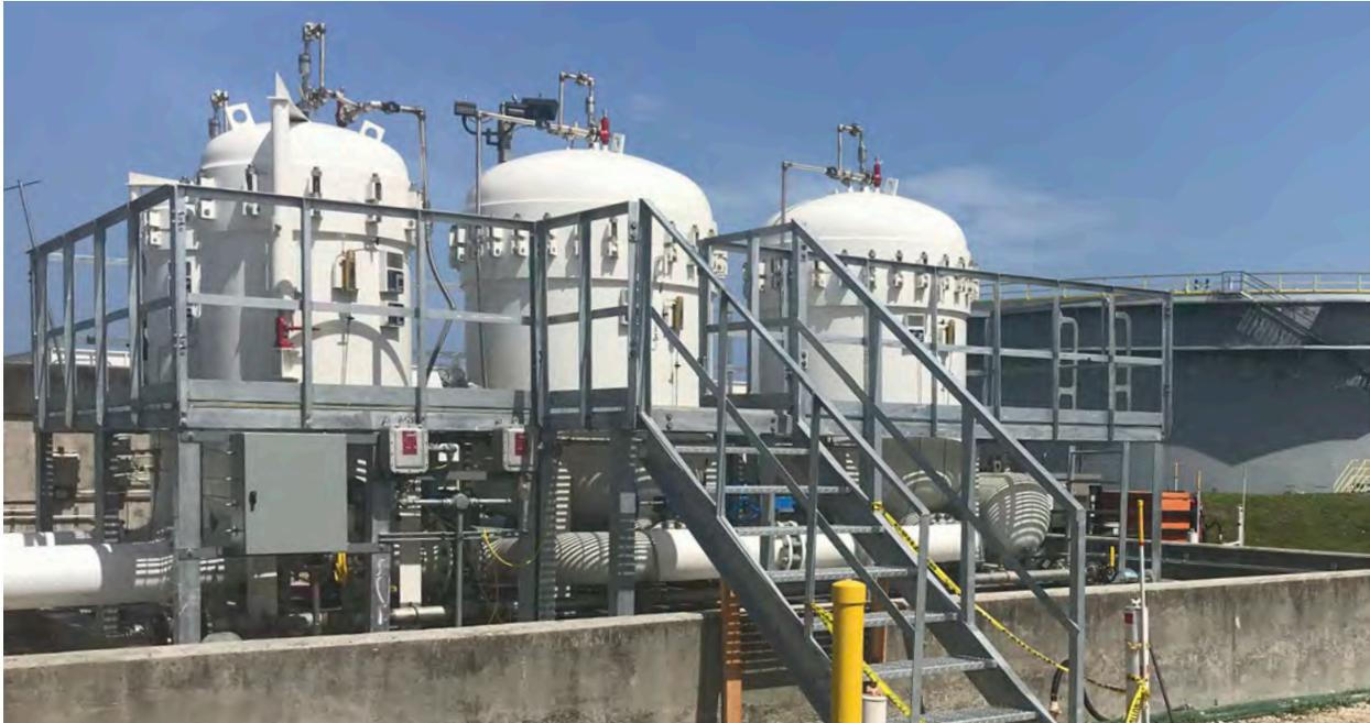
The JFS2500 skid is designed to be a portable, complete filtration system. They can be easily put into service with little more than upstream and downstream connections being made. Great for handling any bulk storage filtration application.
