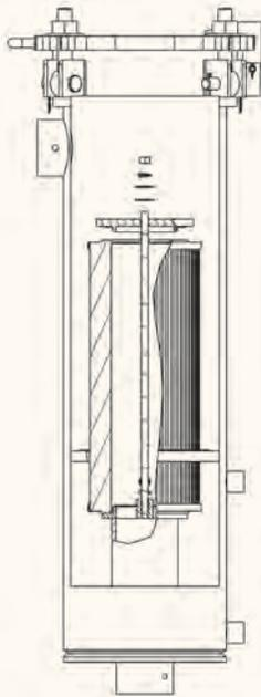
Vel-Max Series with 6" OD x 3.5" ID cartridges can be used in two ways. To remove solid contaminants from a flow stream, use the vessel with a pleated media filter. When used with **Aquacon** cartridges\* the Vel-Max will remove solid contaminants and free water by absorption from a jet fuel or aviation gasoline flow stream.
