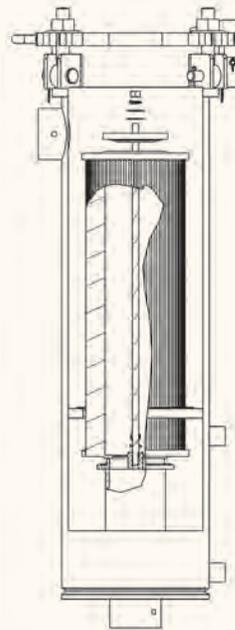
Vel-Max Series for 6" or 6.25" OD x 2.625" ID cartridges can be used in several ways. To remove solid contaminants from a flow stream, use the vessel with a pleated media filter. When used with **Aquacon** cartridges the Vel-Max will remove solids and free water by absorption from a fuel or industrial oil flow stream. Using Vel-Max with clay cartridges will remove surfactants, color and other impurities by adsorption from a fuel or industrial oil system.
