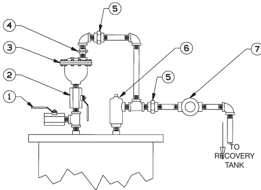
1. Ball Valve – Close for normal operation. Open when filling or draining the vessel.
