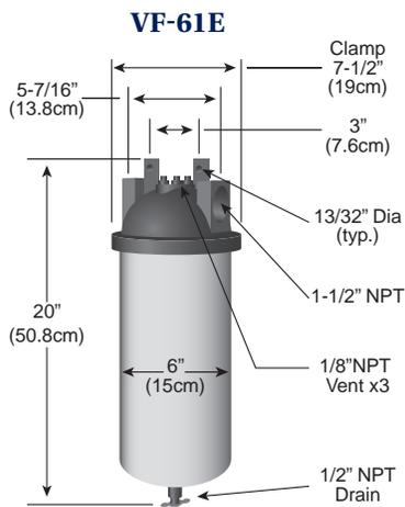
VF-61E has a band clamp closure. Use in areas with limited space.
