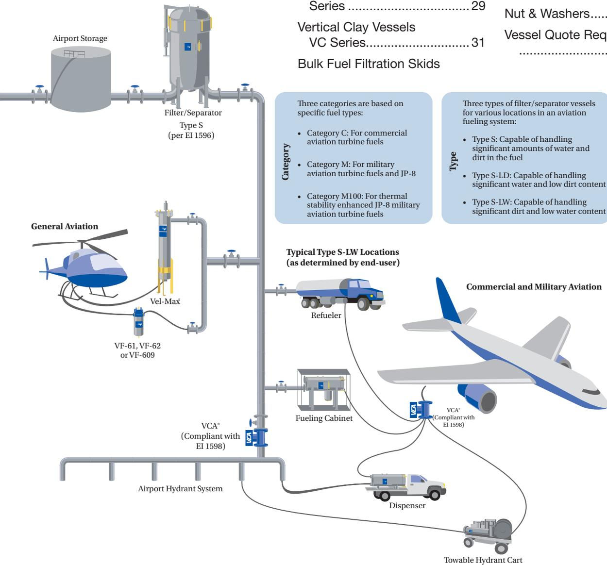
\* Prefilter elements compliance with EI 1590 and vessel compliance with EI 1596 is customer dependent. Optional EI 1583 Qualified Vessels/Absorbent Type Cartridges for jet fuel without anti-icing additive.
