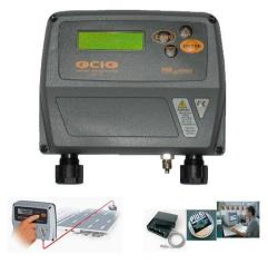
The Piusi OCIO fuel tank gauge is a continuous reading, versatile hydrostatic digital tank level gauge suitable for most fluids. A flexible capillary is inserted into the tank to provide an accurate tank level which is displayed as a percentage, mm, inches, litres or gallons. Predefined high and low-level status alerts will cause the LED screen to flash as standard or two configurable relays allow connection to other equipment such as an audible alarm.
