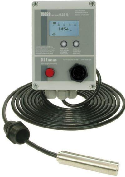
The Ole T5020 is a tank gauge unit that continuously measures the fuel level of your tank. It allows you to read the level remotely via the internet. The Ole T5020 replaces the T4020; offering better accuracy with data and is more affordable. The Ole T5020 is rated weatherproof IP65 (meaning that it is ok to be left out in the rain). It can be calibrated with other Ole products (contact Ole directly for details).
